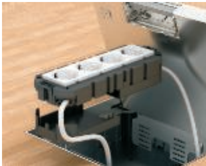
Device mounting in MT module support Devices are mounted in the module support MT3/45 and MT4/45 outside the flush-mount unit. After cable connection, insert the module support into the locking ladders of the flush-mount unit from above.
