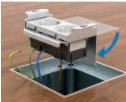
Socket mounting in support Lock the socket in the metal support and connect it. After the connection of the PE cable, bend the metal support through 90°.
