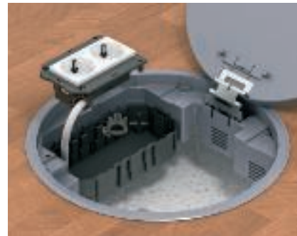
Device mounting in GB mounting box The device is mounted without screws in cover plates and GB mounting boxes. Note: Lock Modul 45® devices into the cover plate for connecting the cable.
