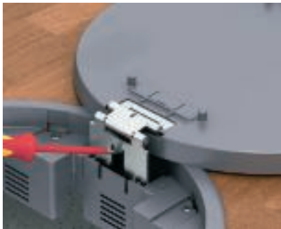
Expansion of the hinged lid for GESR round service outlet Lift the locking lug in the hinge seat of the frame using a screwdriver. Lift the lid out of the holder.
