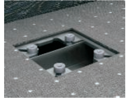
Insertion nut in AIK and AIKA trunking systems Push the insertion nut for the required height into the DAT system opening.
