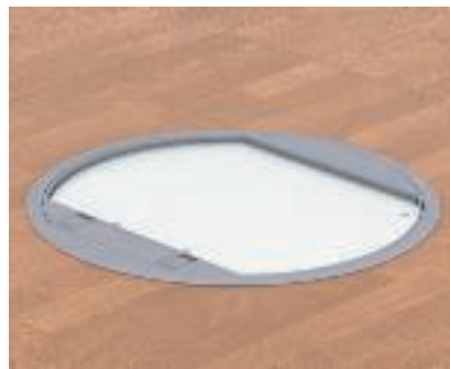
Adjust of the floor covering recess to 3 mm Slacken the 4 lid screws and the inserted 7 mm spacer frame and replace it with the 2 mm spacer bars. Screw the sheet steel lid on again.
