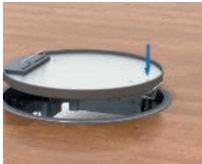
Installation of the hinged lid for GESR round service outlet Insert the lid hinge in the bracket. Press on the lid above the lid hinge until the end position is reached.
