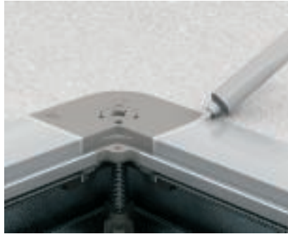
Sealing of the underfloor box with silicone Seal the frame of the underfloor box in the corners using silicone (silicone is included in the scope of delivery of the cassette).
