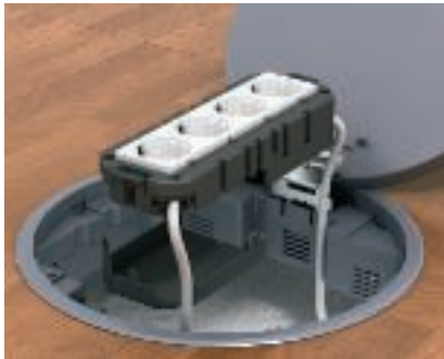
Device mounting in MT module support Devices are mounted in the module support MT3/45 and MT4/45 outside the service outlet. After cable connection, insert the module support into the service outlet from above.
