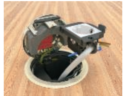
Socket connection Relieve the strain on the connection cable. Connect the socket. Lock the cover plate in the mounting box from above.
