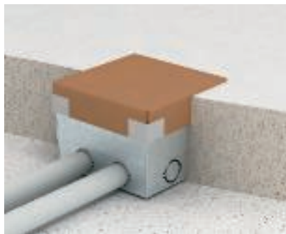
Screed work Lay the screed and work it to the flush-mount unit. Do not use a separating layer.
