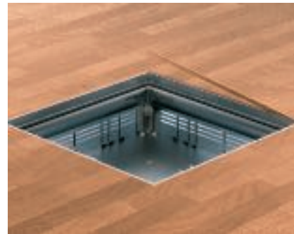
Laying the floor covering on the cassette frames RKS Seal the remaining gap between the floor covering and the cassette frame with suitable materials (possibly with a cork strip).
