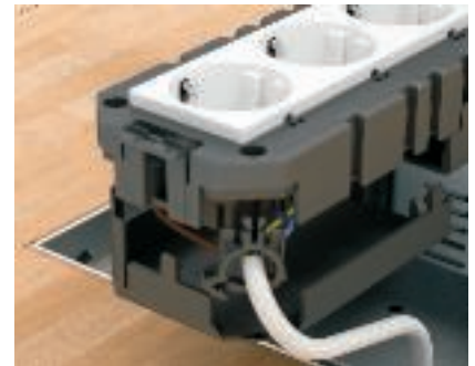
Strain relief for module support mounting Insert the strain relief in the module support from below, insert the connection cable and close the strain relief.
