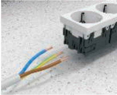
Conventional connection of the socket Run rigid cables to the socket connection. Attach pin-type cable connectors to flexible wire ends.
