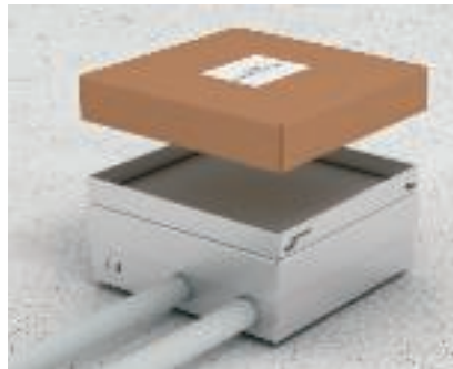
Attach the mounting protection lid Attach the sheet steel mounting protection lid and cover it with a prepared card cover.
