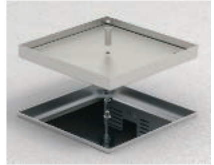
Mounting of threaded sleeves This work step takes place before the floor covering is laid in the cassette. Drill a fastening hole for the threaded sleeve (Ø 8 mm). Insert the threaded sleeve and fasten it.
