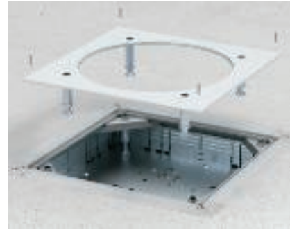
Preparation of an underfloor system Mounting the heavy-duty blanking lid on the underfloor box. Adjust the support feet to the right height and secure with a locknut.
