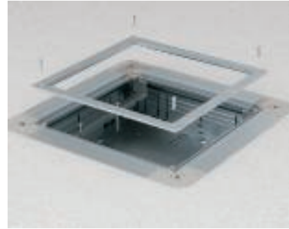
Installation of blanking lids Fasten the blanking lid on the underfloor box. The levelling profile must be visible in the mounting opening.
